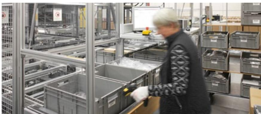
Laser-guided and visually supported picking in the automatic small-parts storage area
