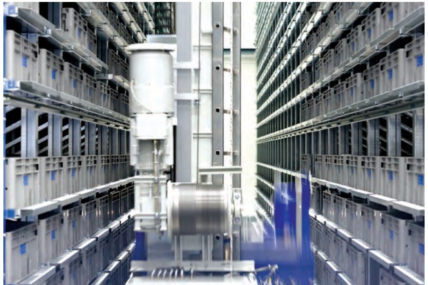
[ Automated storage and retrieval machines weigh a lot less than aisle trucks ]
