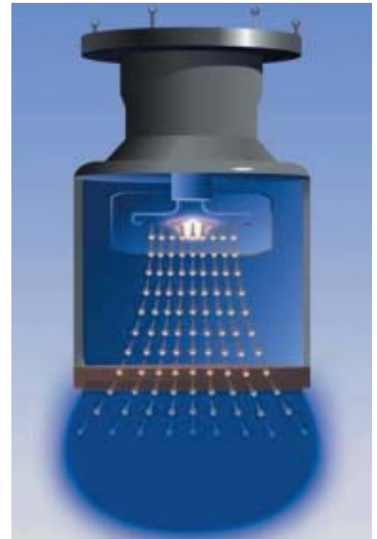
The emitter produces a cloud of energy, which is a fast and effective method for surface sterilisation.
